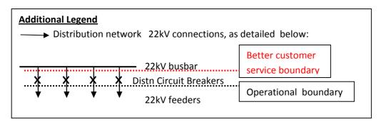
The current inappropriate operational boundary requires Distribution operator to request help from Transmission operator to deliver service to retail customers, both for routine daily work and maintenance, and to restore supply following a fault in the distribution network.
